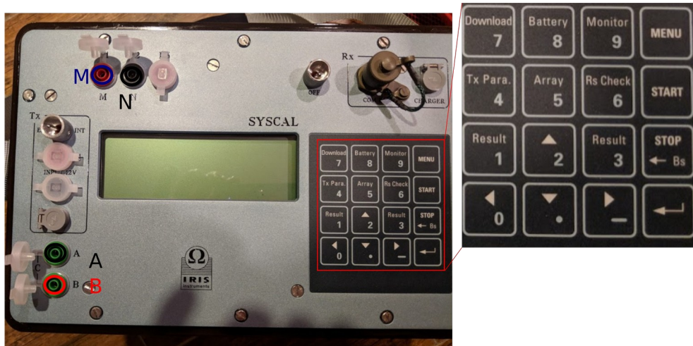
Figure 1: Syscal R1+ front panel showing the proper connections. Inset shows the keyboard panel .
