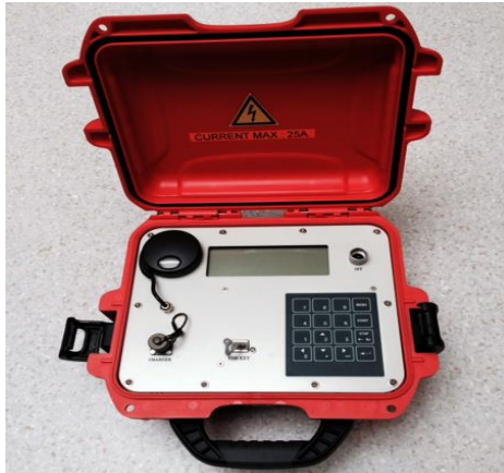
I-Fullwaver, compact recorder for full wave signal
